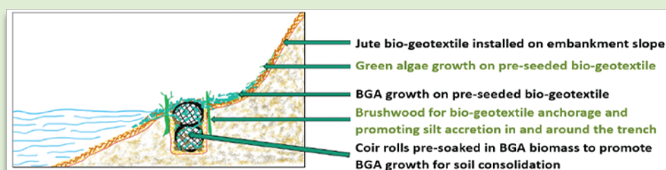
Figure - 13. Proposed methodology of digging trenches to fit in the overlaid bio-geojute textile and secure it with brush wood and coir rolls soaked in blue green algal biomass to trigger blue-green algal growth to consolidate the soil faster.
