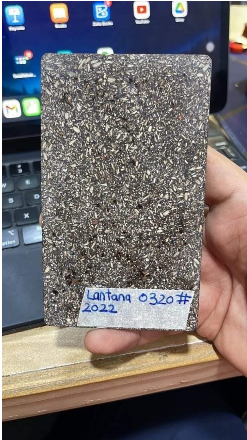
Finished Lantana plywood
