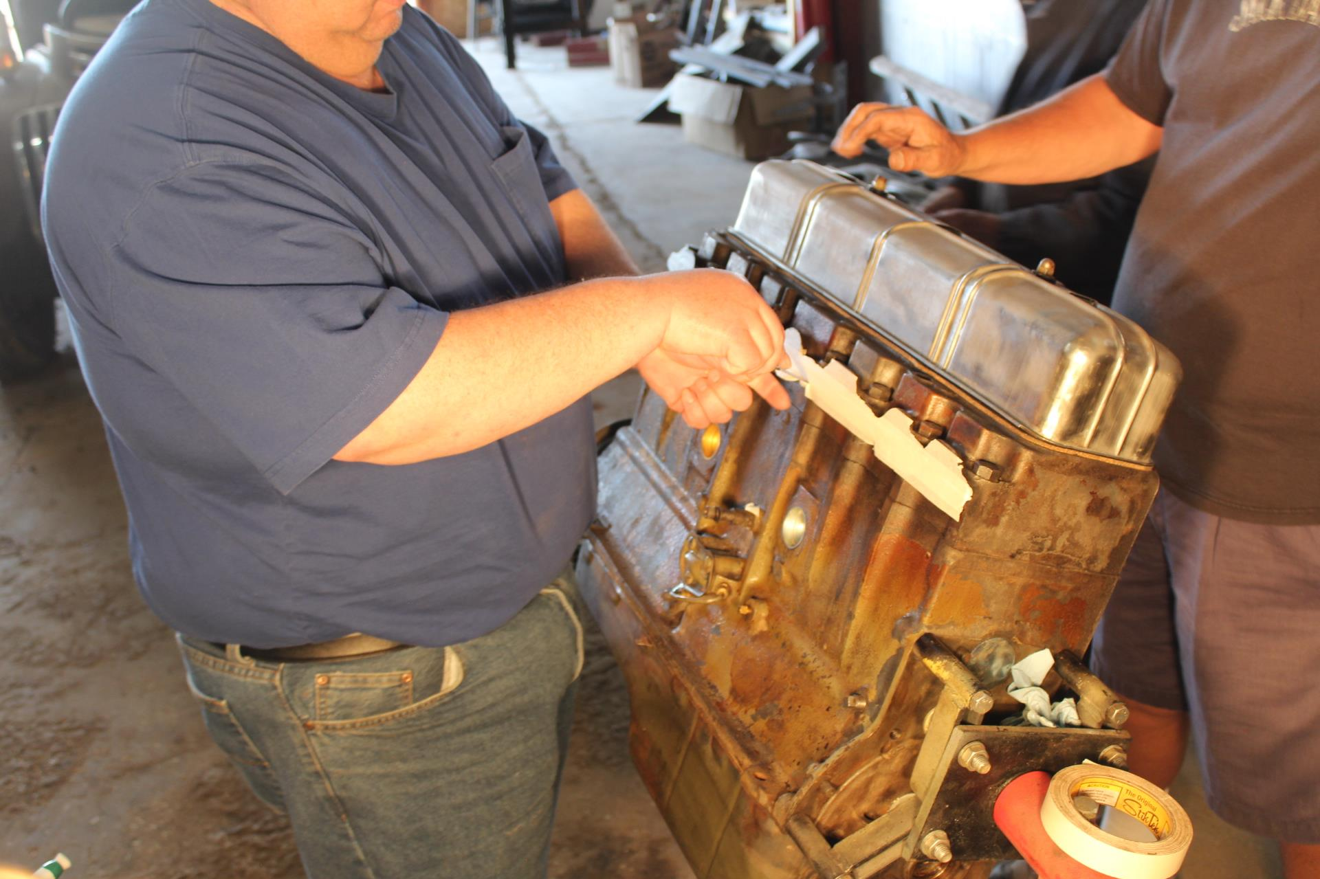
John Gudgeon masks off the intake and exhaust ports prior to painting..
