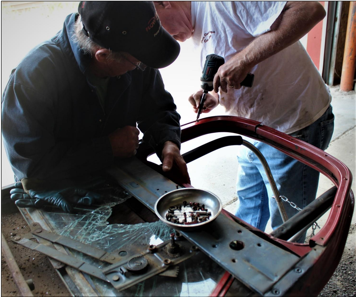
Mike Johnson and Mike Kennedy disassemble the 1942 drivers side door. They successfully removed the window and frame.
