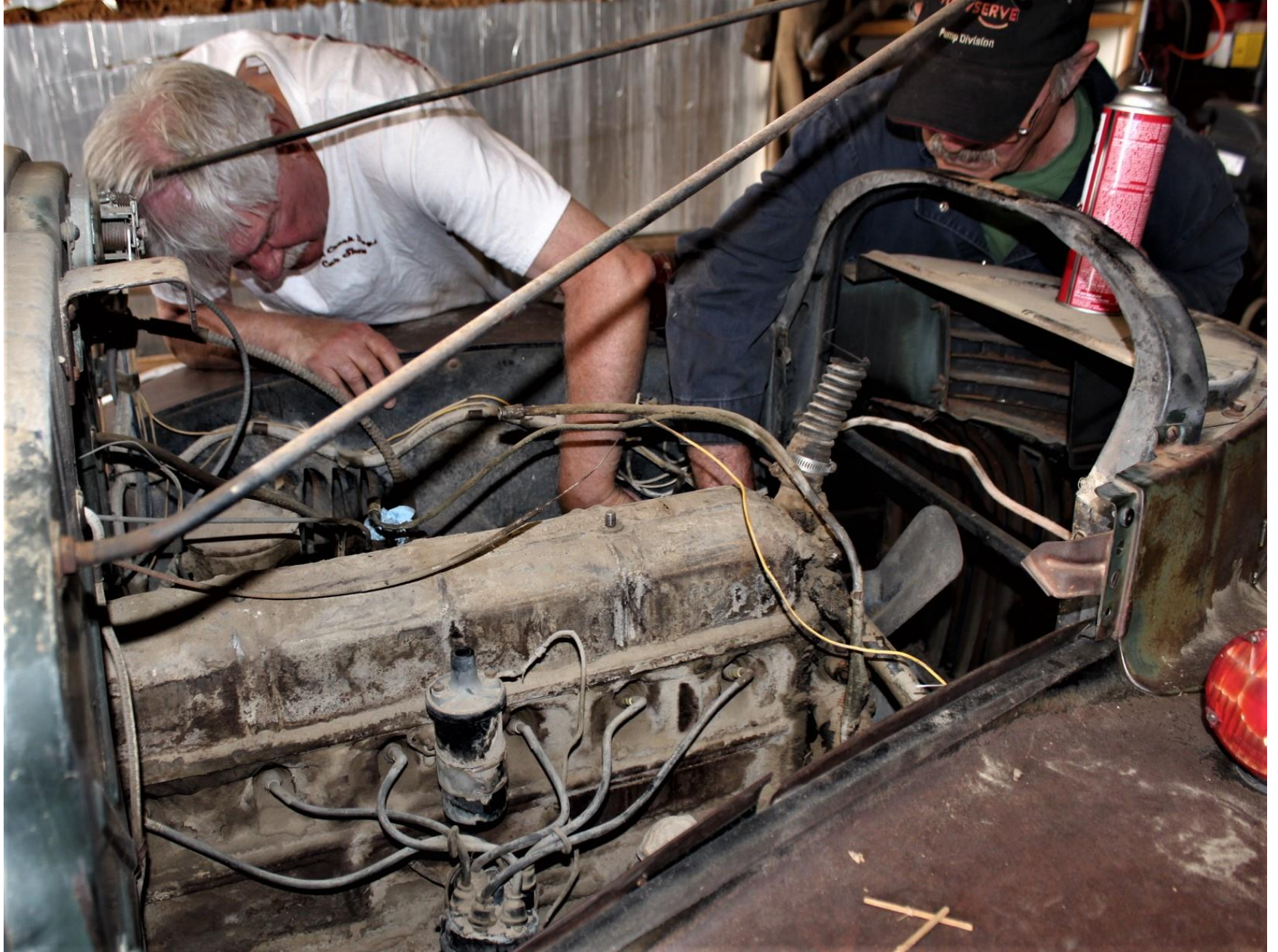
Mike Johnson and Mike Kennedy retrieve the 1941 generator bracket.
