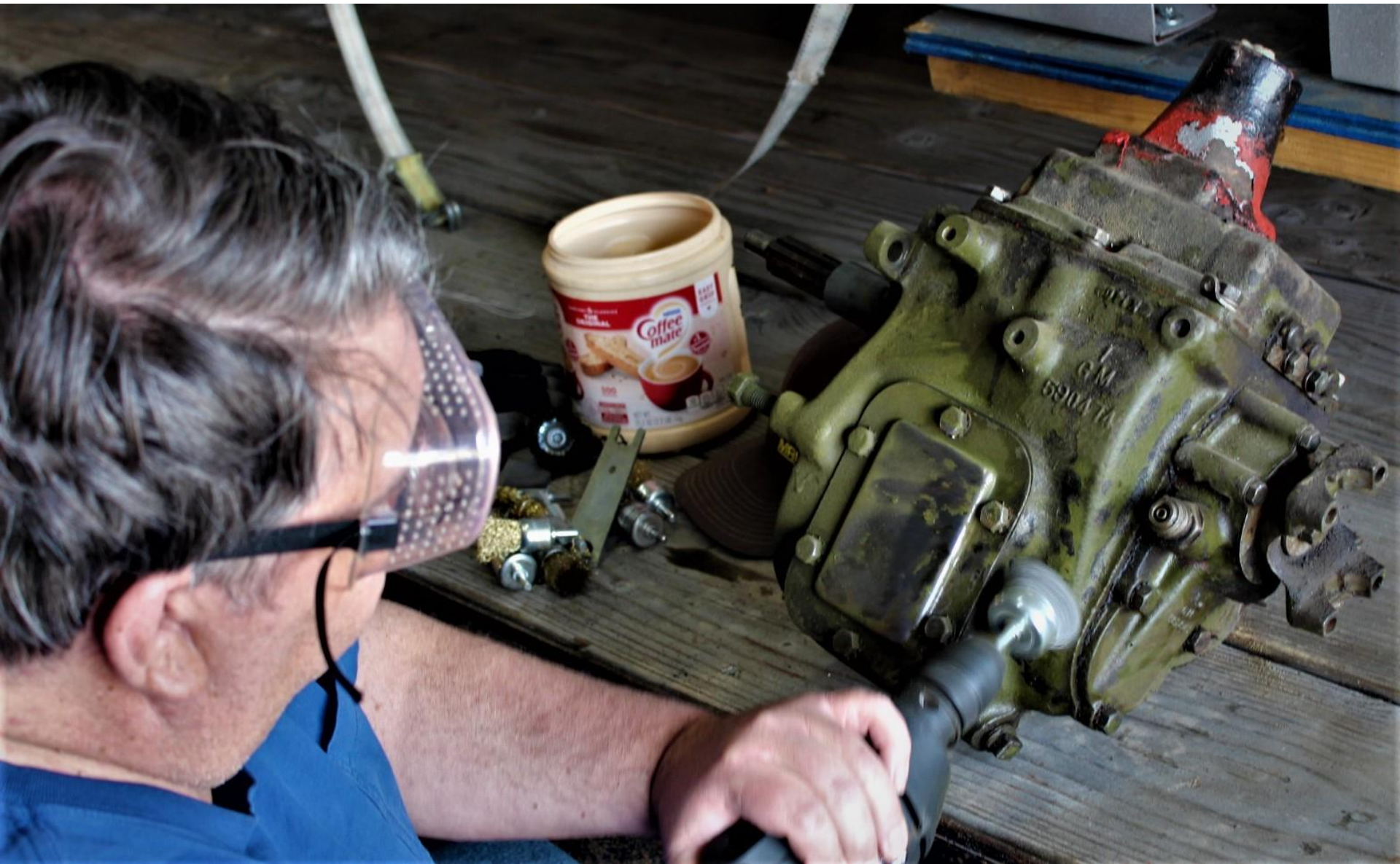
John Gudgeon drew the task of cleaning the transmission. The gears seem to be in good condition.
