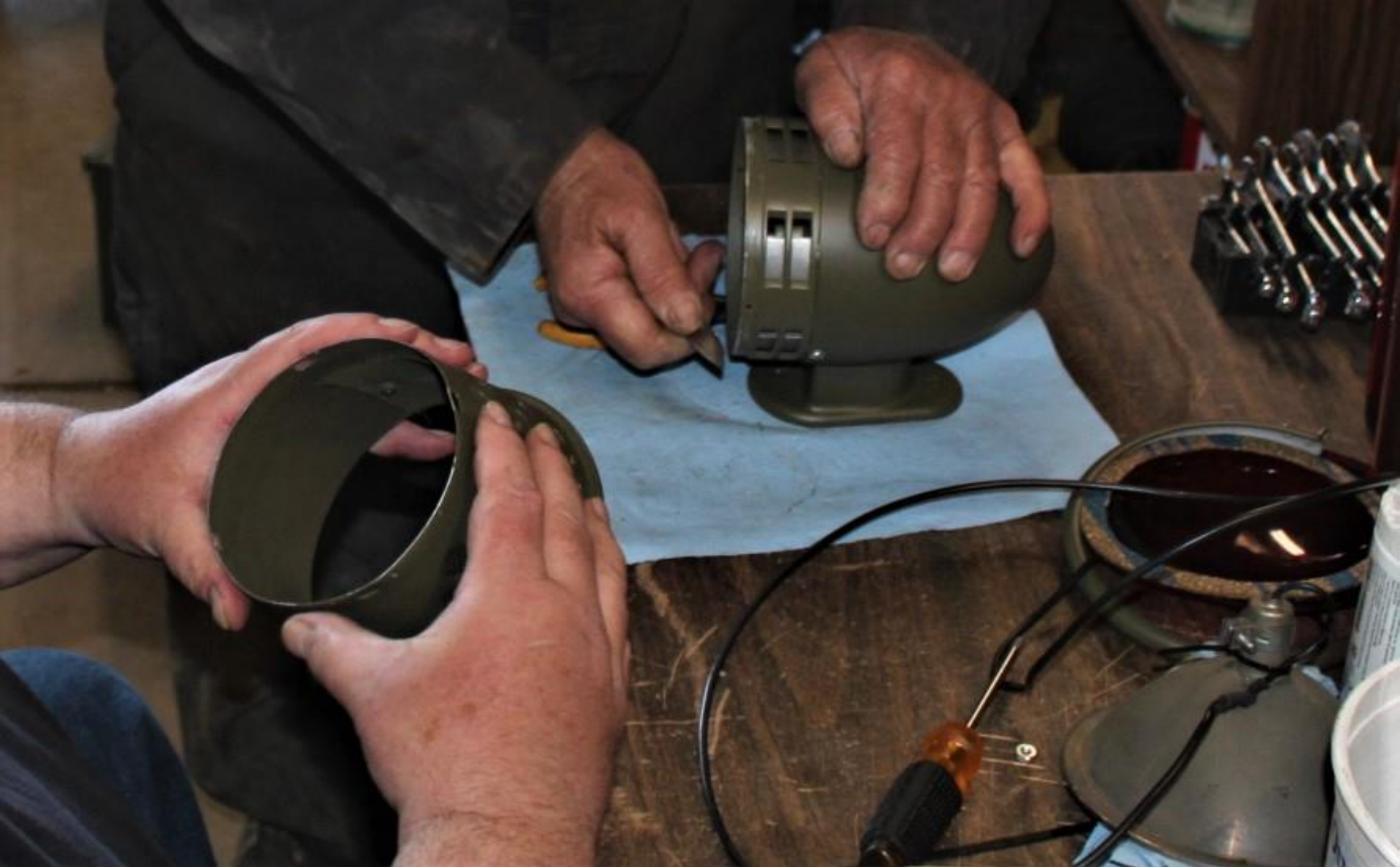
Siren and light modules are being assembled by Mike Johnson and John Grudgeon. The electrical components were restored earlier. Doug Walters painted the cases. The siren is as loud now as when it was new.
