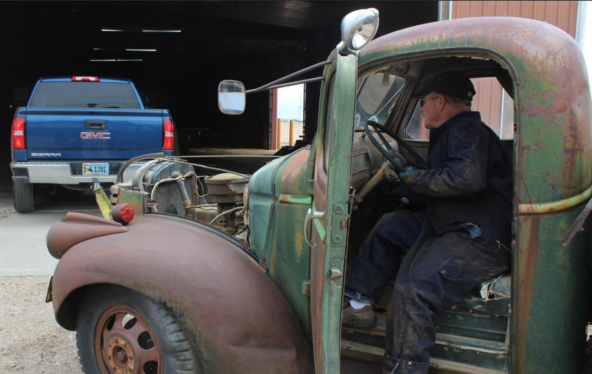
The 1941 truck is mostly complete and original, and will provide needed parts for the fire truck. It will also serve as a guide for restoration, since the fire truck has many modifications from factory original.
