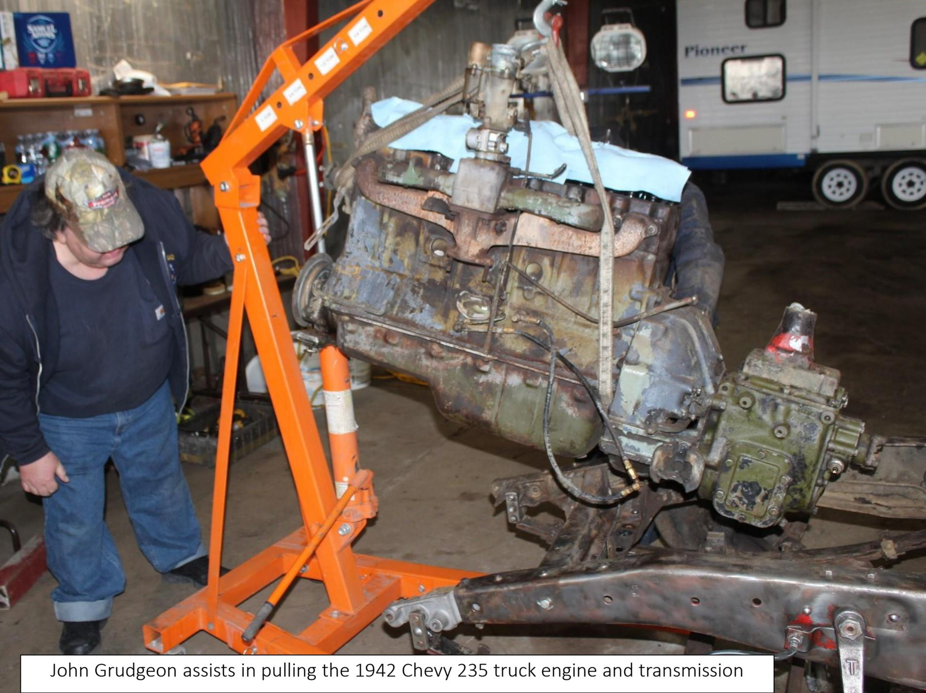
John Grudgeon assists in pulling the 1942 Chevy 235 truck engine and transmission
