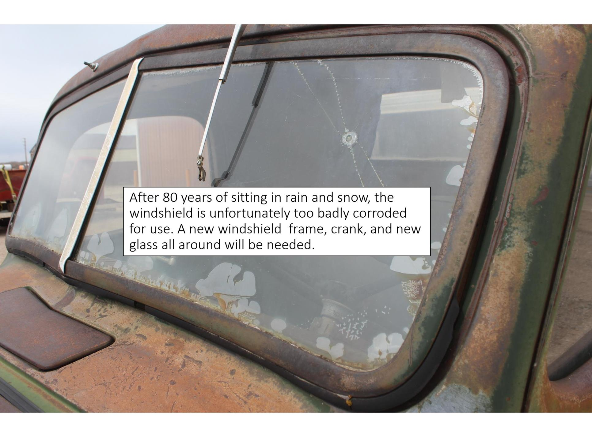
After 80 years of sitting in rain and snow, the windshield is unfortunately too badly corroded for use. A new windshield frame, crank, and new glass all around will be needed.
