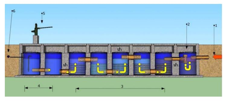
Schematic Diagram of IHome-WV Wastewater Treatment System.
